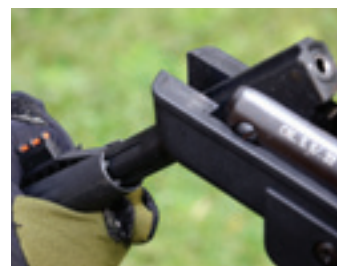
The barrel sleeve makes cocking easy
